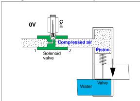
Here, there is no tension though the spool and the solenoid valve is held up by the force of the spring. This means that compressed air affects the water valve's piston and the water valve closes.
