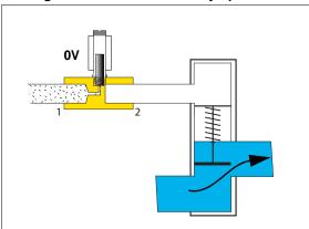
Here, there is no tension though the spool and the solenoid valve is held down by the force of the spring. This is so that no compressed air reaches the water valve's piston. The water valve is now open, which is its position unaffected by compressed air.
