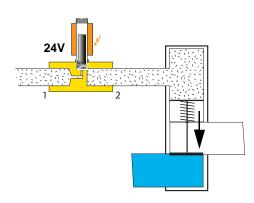
Now, the spool is fed with voltage which means that the solenoid valve opens and compressed air reaches the water valve's piston. The water valve is then pushed down and closes the water flow.
